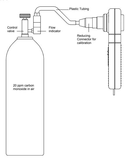
The plastic tubing supplied with the gas should be pushed firmly over the reducing connector.
