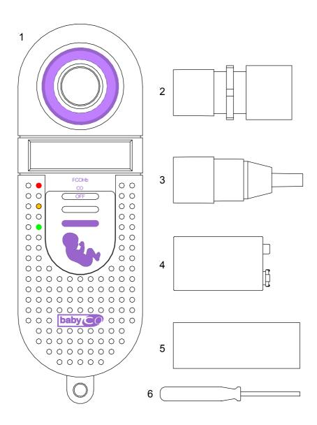
The CO sensor is an electrochemical fuel cell, and works through the reaction of carbon monoxide at one electrode and oxygen (from ambient air) at the other. This reaction generates an electrical current proportional to the concentration of CO exposed to the sensing surface of the fuel cell.
