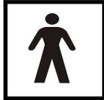
Definition: Type BF equipment – equipment providing a particular degree of protection against shock, particularly regarding allowable LEAKAGE current and reliability of the protective earth connection (if present).
