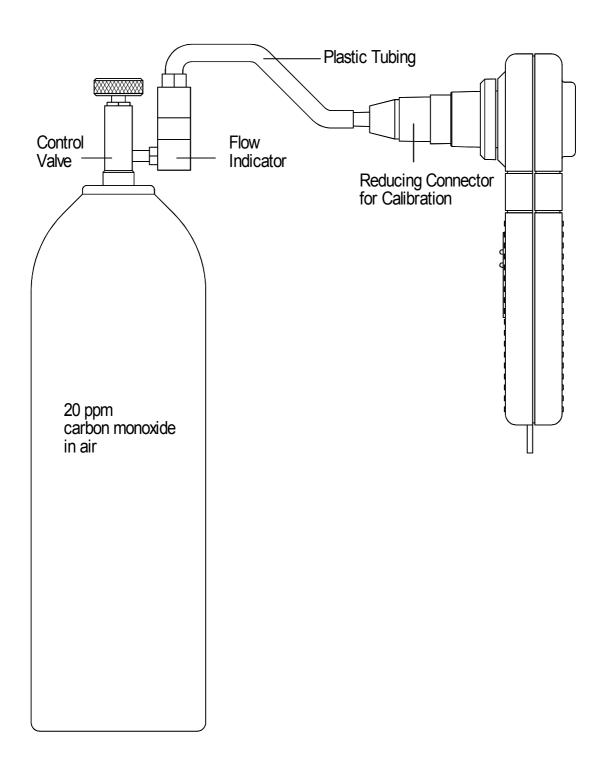
1. Set up the calibration equipment as shown above.
